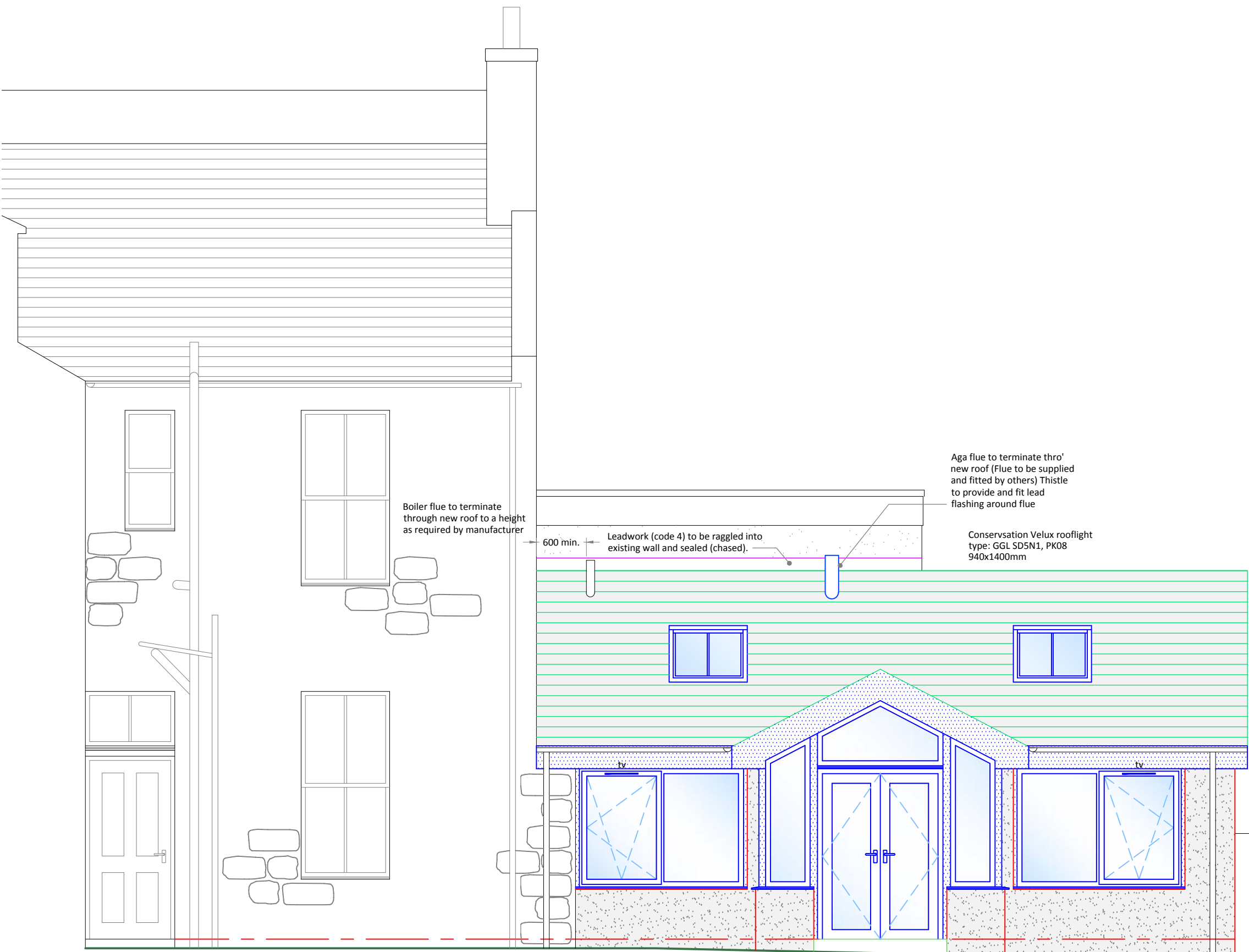
Proposed South Elevation (1:50) New french doors and glazed pane either side to have laminated glass outer panes
